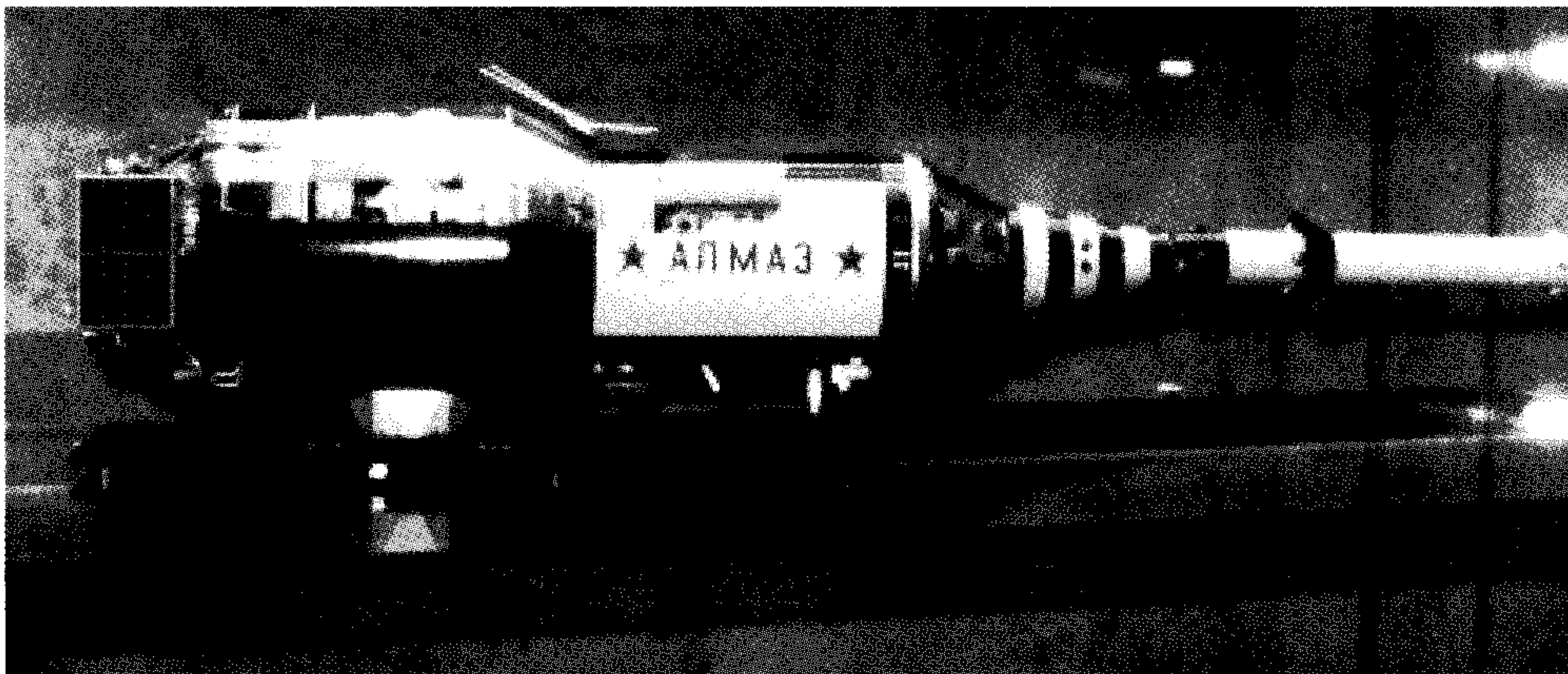
Fig. 2 This is a model of the original Almaz Orbital Piloted Station (OPS). On the right is the conical Return Apparatus (VA) with its launch escape tower. The middle area (with the word "Almaz" written in Cyrillic) is the living quarter of the station. The larger diameter section on the left contains the photo-reconnaissance camera system known as Agat-1. A Soyuz would dock on the left port of the station, with the crew entering the station into the large diameter area.
